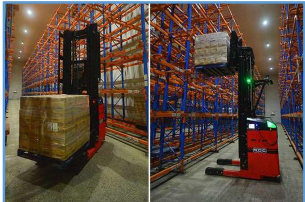
Pallet picked and ready to put away (left), the AGV expertly placing the pallet on the racking.
